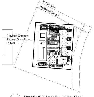
L23 Rooftop Amenity - Overall Plan See Sheet 05 \* THE PROJECT UTILIZES ALL YARD REQUIREMENTS FOR THE C2 ZONE (LAMC 12.14C) IN ITS COMMERCIAL PORTION (PARKADE & GROUND FLOOR LEVELS) AND R5 ZONE PER LAMC 12.12.C AND LAMC 12.22(C)(3) IN ITS RESIDENTIAL PORTION.
