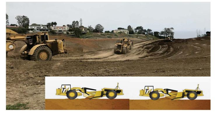
Scrapers are capable of massive grading operations by picking up layers of soil a few inches thick over a long length of haul and so inherently require a large amount of earthwork for access roads and maneuverability. This means that small adjustments in excavation depth may result in relatively large grading areas. With as many as 7 scrapers on the job it is not cost effective to put them on hold while smaller more precise equipment removes the unsuitable soil/debris/mud.
