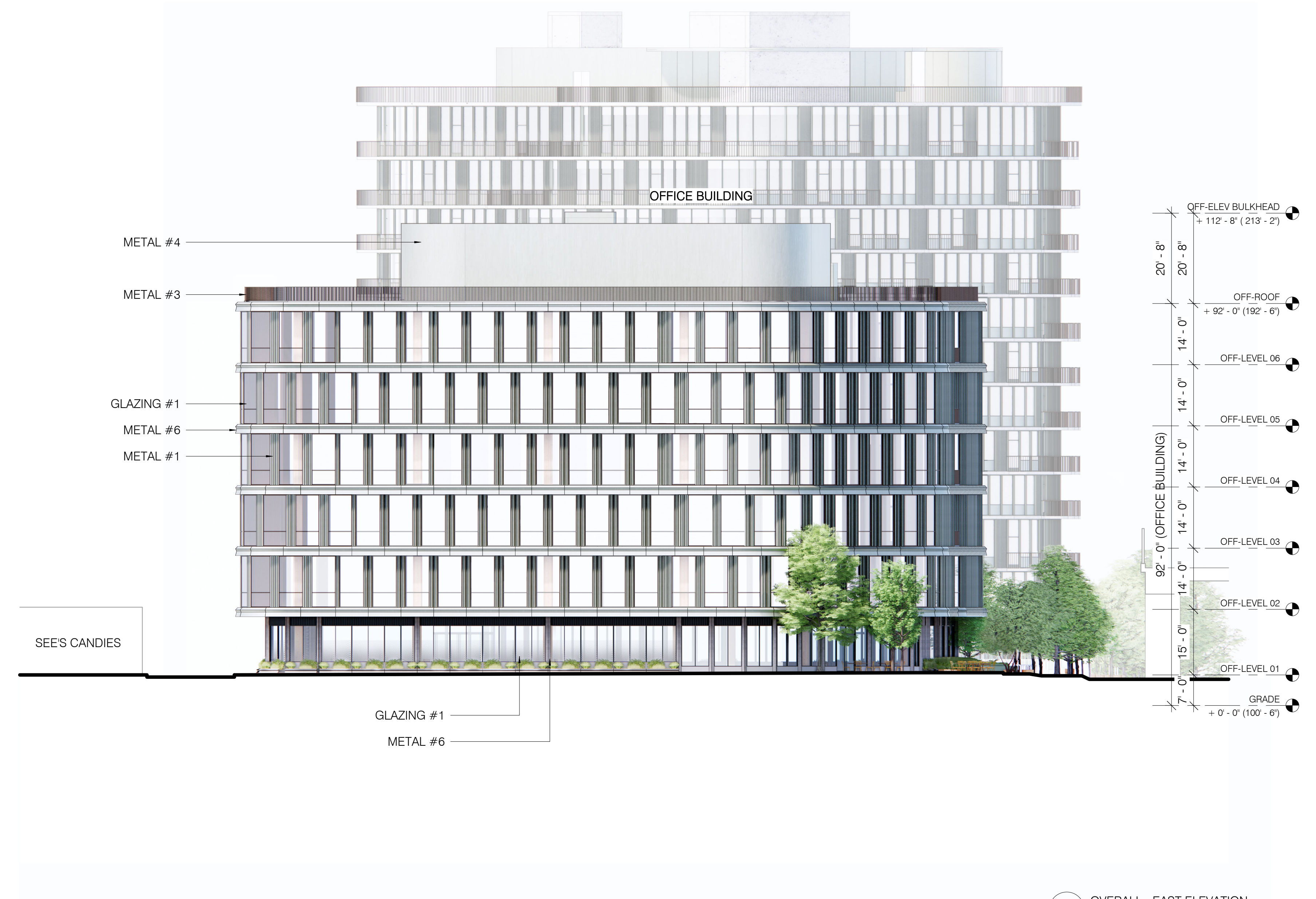
2 OVERALL - EAST ELEVATION 1/16" = 1'-0"
