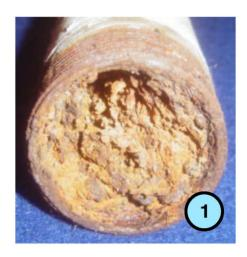
Detail of clogged and rusted pipes from the Pool Repair sketch–an example of the problem at Granada Hills
